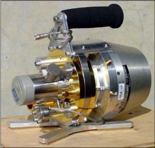
Courtesy/Lawrence Berkeley National Laboratory This portable radiation detection device, known as Cryo3, is able to distinguish between harmful and benign forms of radiation.
